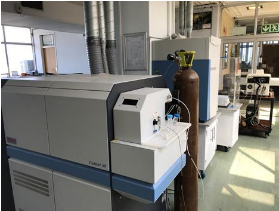
Perkin Elmer Elan DRC-e ICP-MS (previous page) and Thermo Element XR (above) at the Earth Lab, Wits University.
