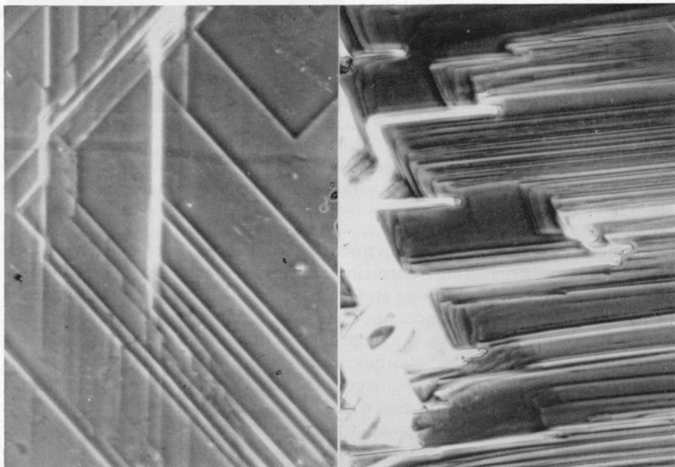
FIGS. 5 and 6: FIG. 5 (left). Slip lines formed during crystal growth. (10\bar{1}1) face of natural quartz, Kurobira, Kofu, Japan. Positive phase contrast. \times 160 . FIG. 6 (right). (10\bar{1}0) face of natural quartz. Positive phase contrast. \times 160 .
