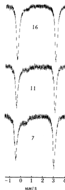
Figure 1. Mossbauer spectra of pyrope and almandite. No. 7, pyrope from kimberlite; No. 11, pyrope from the mantle-derived xenolith; No. 16, almandite from metamorphic rock.
