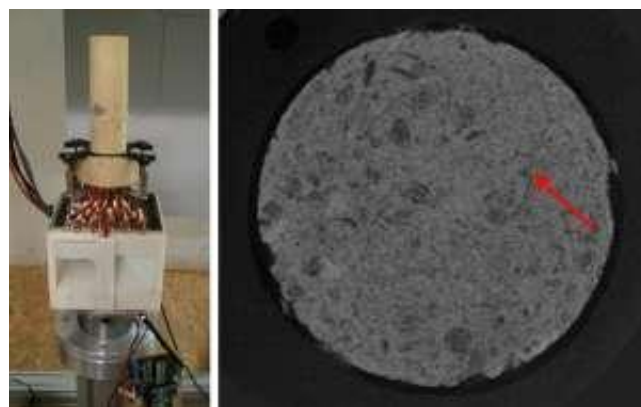
Figure 1: Custom made freezing cell (left); transversal slice with scaling crack (right).
