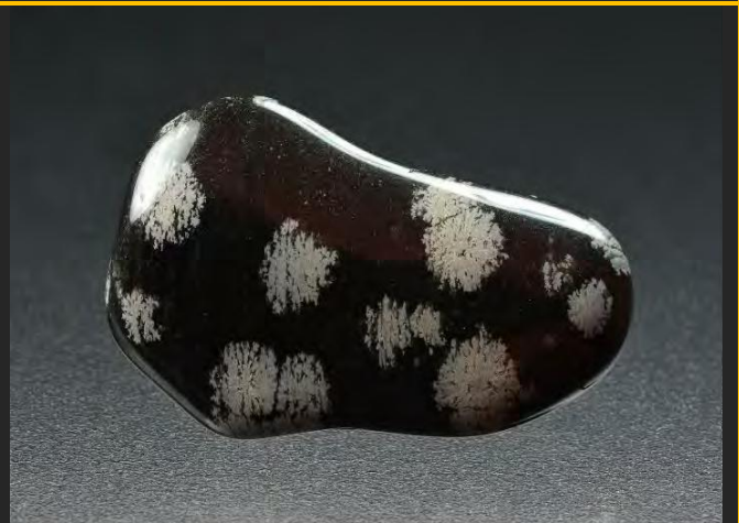
"Snowflake" obsidian. A small 3.2 cm tumbled and polished specimen. The "snowflakes" are cristobalite, formed during the partial crystallization of the volcanic glass – see https://www.mindat.org/min-8520.html Black Spring, Black Rock Desert, Millard County, Utah, USA.
