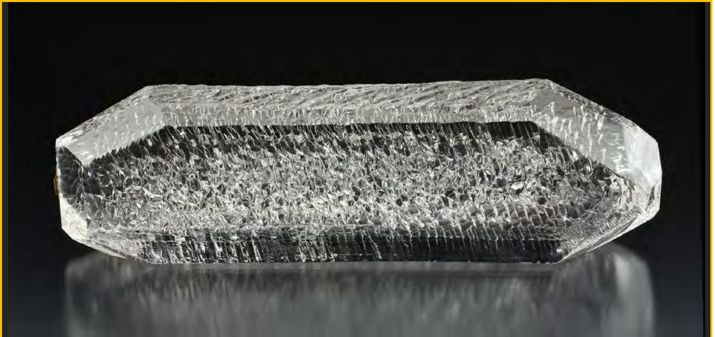
The final picture is of a glassy, synthetic quartz crystal. This is 22.1 cm long and was grown from a seed crystal in an autoclave at STC (Standard Telephone & Cable) located on the East Rand, Gauteng, under temperature conditions of 300-400 C° and pressures of 130-145 Mpa. These ultra pure crystals are used to manufacture silicon chips. See this link to see how they are manufactured: https://www.ndk.com/catalog/AN-SQC_GG_e.pdf .
