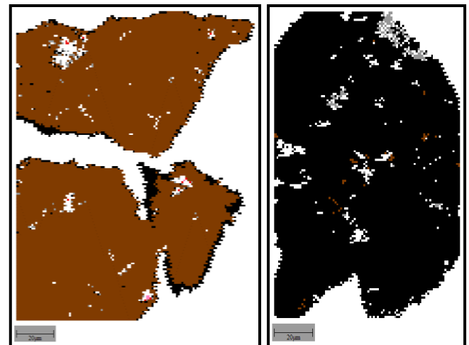
Figure 4: Top: Image of hematite (left) and magnetite (right) mineral standards used for the study. Left: AMICS measured hematite standard. Right: AMICS measured magnetite standard. Brown: Hematite, Black: Magnetite, Grey: Other.
