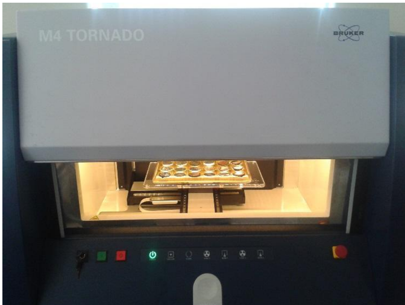
Figure 6: Oblique chamber view of Bruker M4 Tornado. A “Ferrero Rocher” chocolate box is present in the chamber with 24 30mm diameter sample standards. The box represents an area of approximately 18 by 24 cm, all of which can be accessed with the stage movement and as such all of which can be measured and seen by the detectors.
